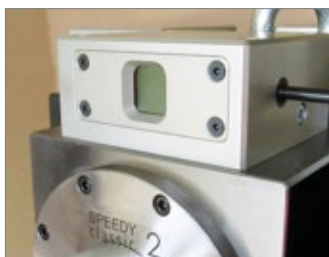
The green indicator indicates correct clamping.
