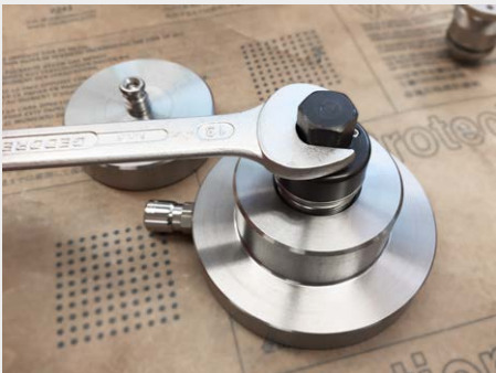
Tighten with mounting key (15 Nm)
