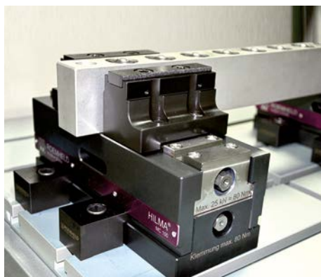
Clamping of aluminium bars with workholding system HILMA.MCP 100 Z Balance.
