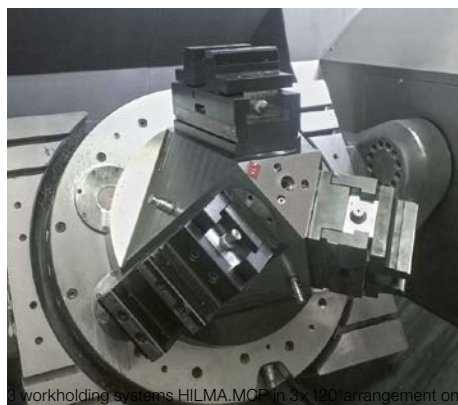
Workholding systems HILMA.MCP in 5-axis arrangement on a 5-axis machining centre.
